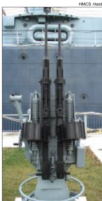
Twin Oerlikon 20mm mount as displayed adjacent to HMCS Haida .
